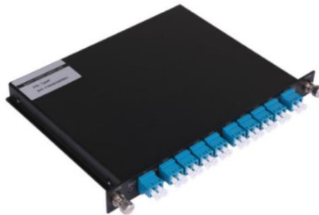
An example of a CWDM multiplexer and demultiplexer in a KAS cassette housing
